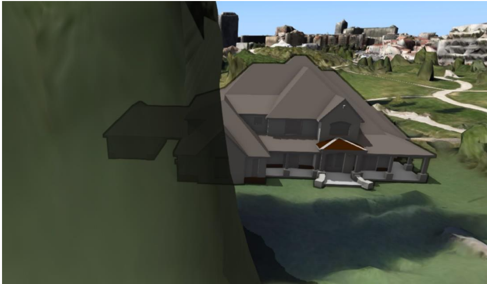
Figure 4: Parts of the building hidden by terrain or other structures are shown as a visual aid for planning.
