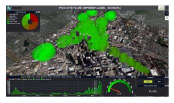
This example is similar to a CBRN plume release of mustard gas or smoke from a fire in an urban environment. This models the dispersion of the smoke over time and indicates the density of the gas at elevation and on the ground.
