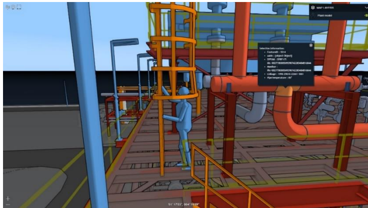
Figure 5: The “Selection on OGC 3D Tiles data” sample illustrates how to color pipe segments based on real-time temperature measurements.
