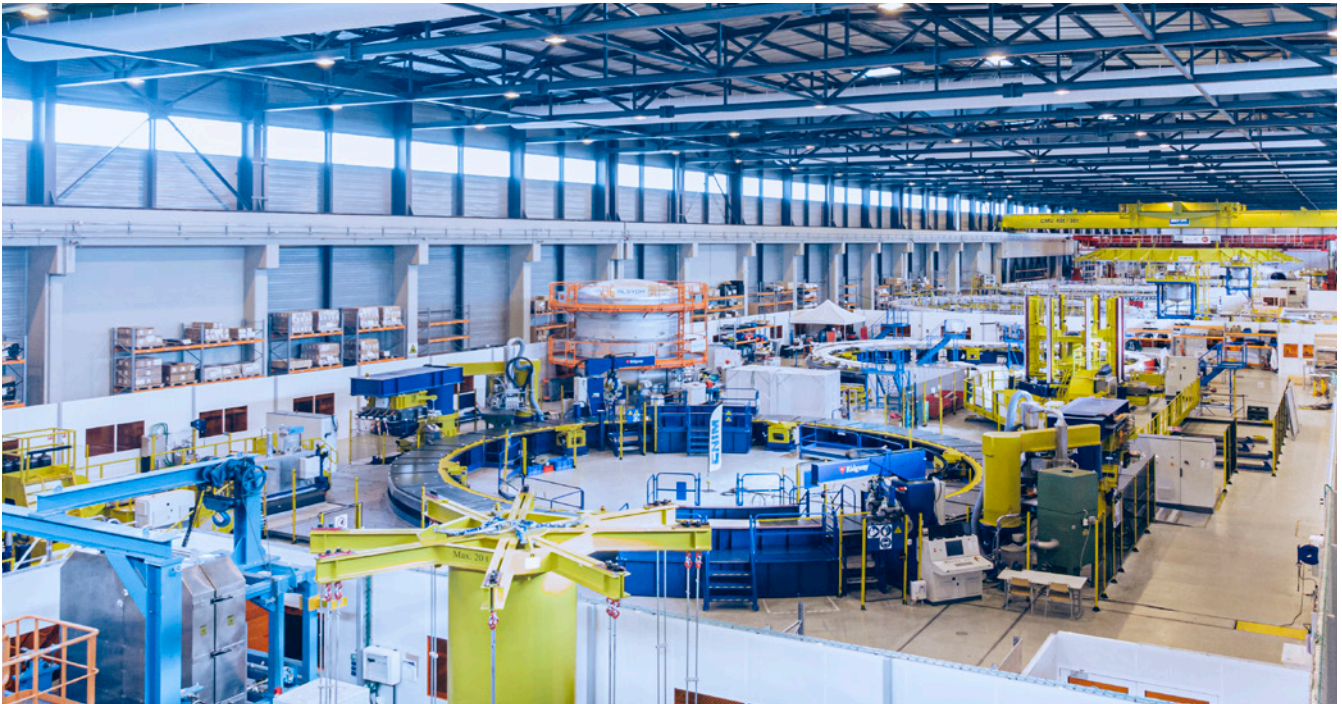
View of ITER Poloidal Field coils factory on-site, where four of the five coils that Europe is responsible for will be manufactured. © F4E
