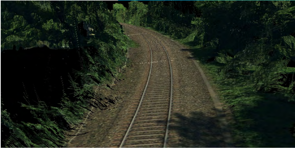
Point cloud created using SGM correlation from 2 cm GSD DMC imagery.
