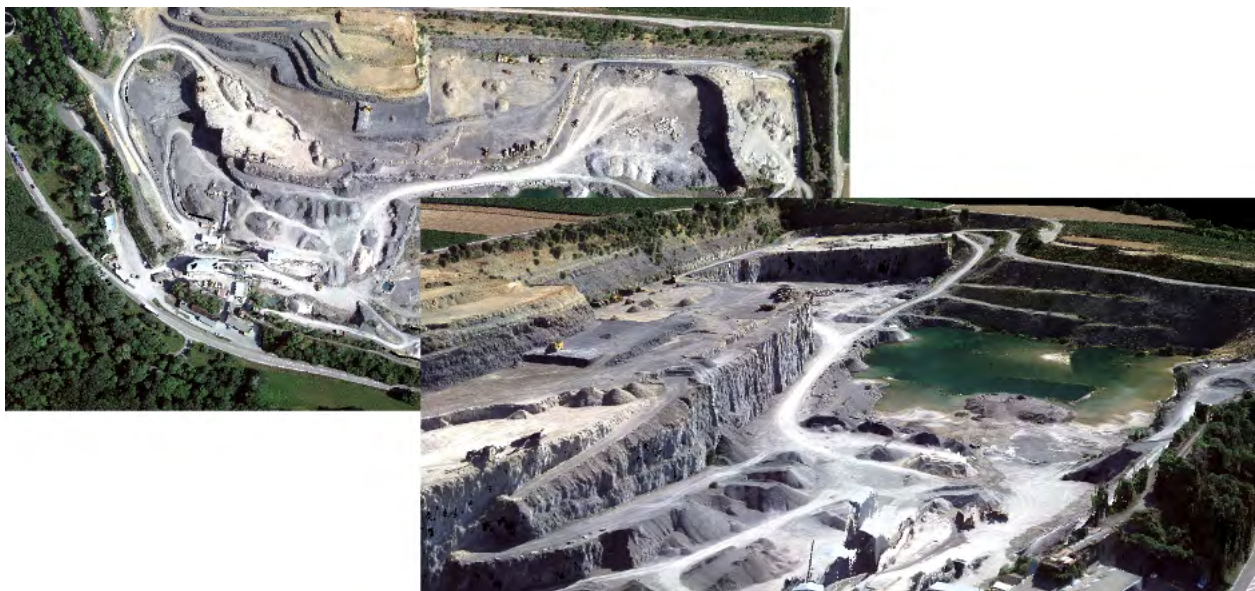
Top-down and iso views of point cloud created using SGM correlation from 10 cm GSD DMC imagery.
