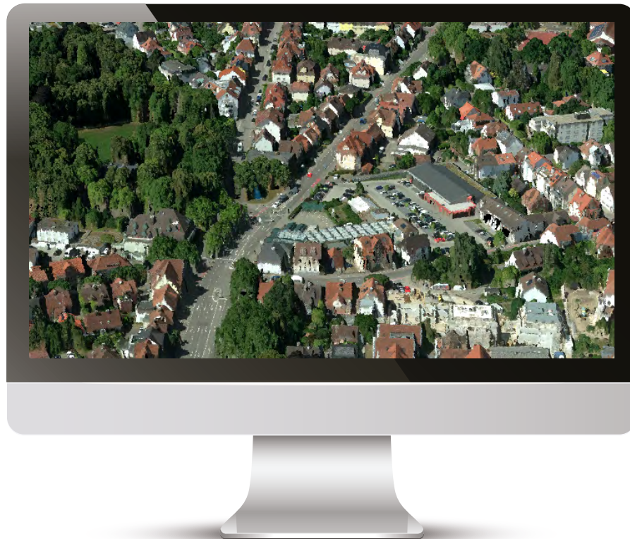
Point cloud created using SGM correlation from 5 cm GSD DMC imagery.
