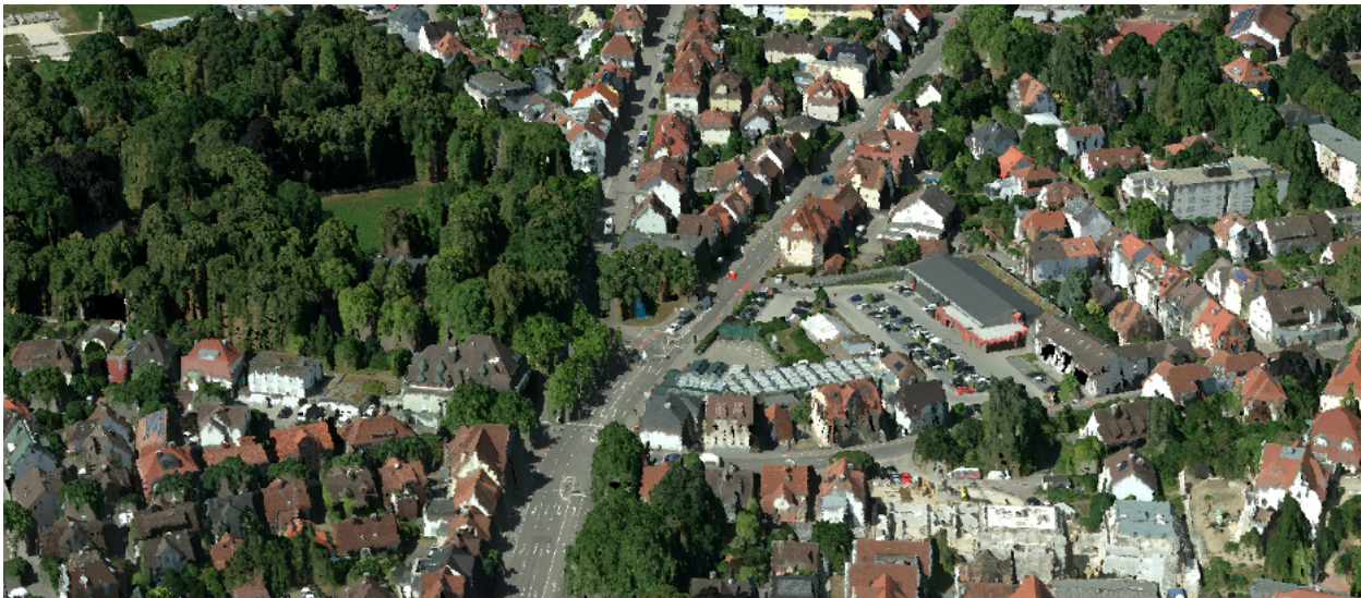
Point cloud created using SGM correlation from 5 cm GSD DMC imagery
