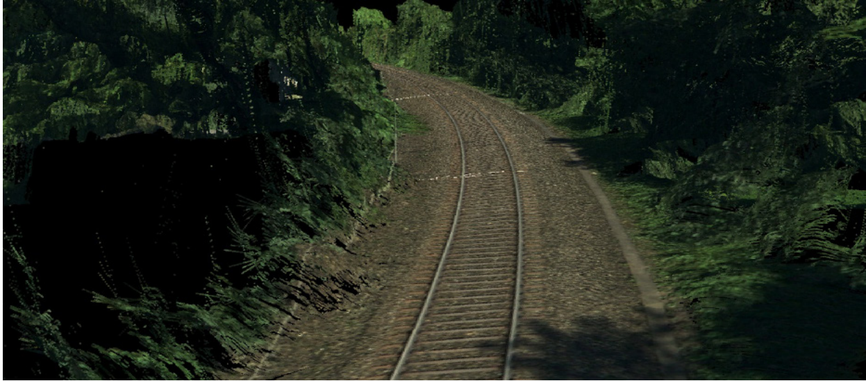
Point cloud created using SGM correlation from 2 cm GSD DMC imagery
