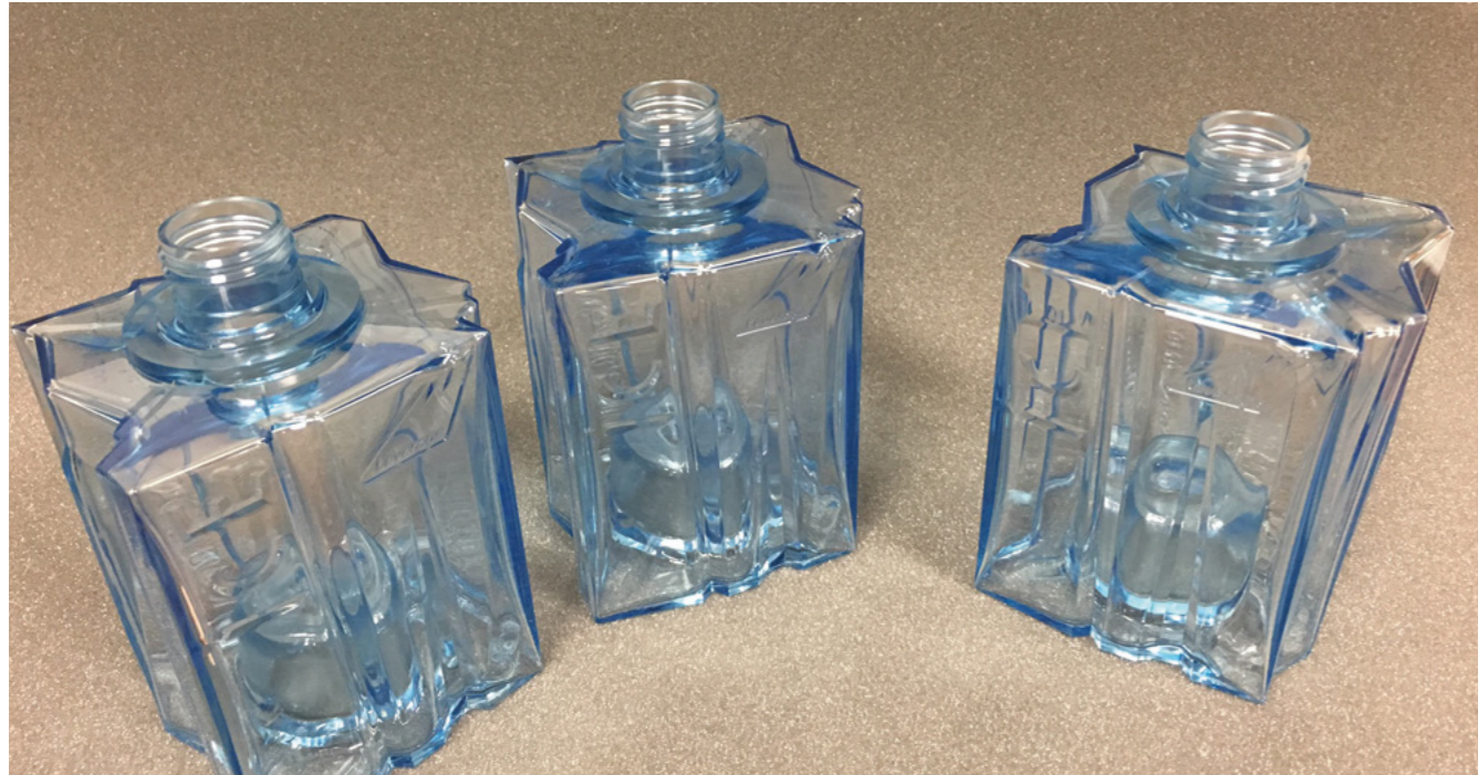
Bottles produced on one-stage injection stretch blow machines using mould tools created with EDGECAM and WORKNC.
