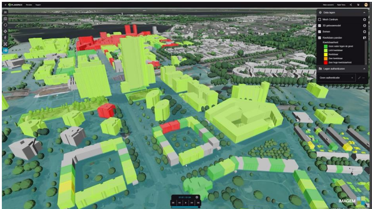
Hexagon partner IMAGEM's flood prediction solution: buildings in red are at risk of flooding in the simulated scenario.
