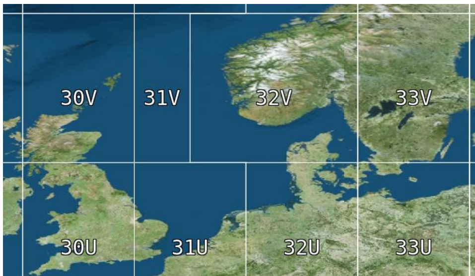
Figure 2: A MGRS grid overlaid on a LuciadRIA 2D map view, illustrating zones, grid cells and their labels
