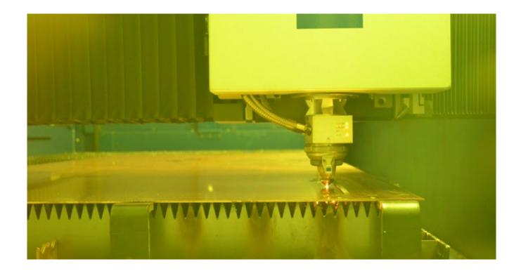
The other key area for them is around the electric motor itself, producing specialist products both for the drivetrain and in-wheel. While most of their parts, both for busbars and motor laminations, are cut from sheet material on a Trumpf laser CNC machine tool, programmed with the industry-leading RADAN CAD/CAM software, they also use wire erosion, mainly for prototyping and developing small series production.
