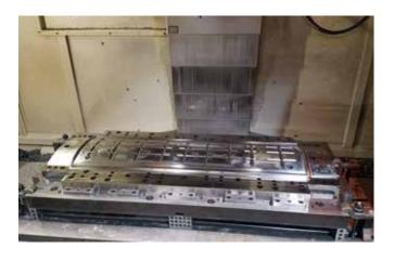
Planar toolpath is designed to machine in parallel passes following the surface profile of the part, with a constant stepover in the plane view. Z-level finishing toolpath is most helpful when machining parts with vertical or significantly curved shapes and is particularly adapted for use with bull-nose cutters on all kinds of materials.
