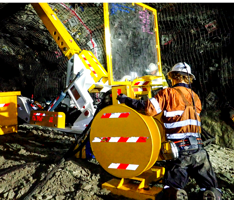
Figure 3. View of Beltor's MED with the operators underground, in the process of retrieving the LH621 loader in Australia.
