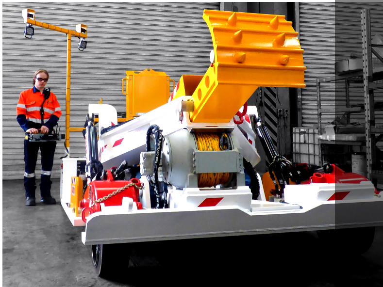
Figure 2. Mine Extraction Device (MED) converted for use with HARD-LINE's Radio Remote Control (RRC), equipment operator shown on the left.
