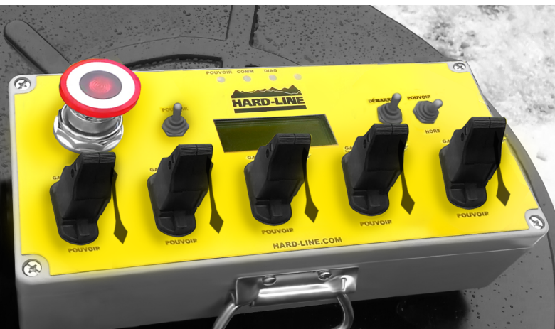
Figure 1. A fully customized RRC Remote was built to use with Beltor's MED. Below is a recreation of the remotes layout and components.
