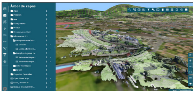
CAR Cundinamarca’s geoportal: An integrated 3D visualization of point clouds, digital terrain models and orthophotos, leveraging M.App Enterprise, Luciad and ERDAS APOLLO
