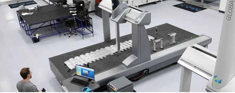
The large and complex parts often dealt with by Max Aerostructures would requiring an full working day of inspection time on the CMM, and that only after the creation of an intricate measurement program – with the HP-L-10.10, this workload can be reduced to just 7 minutes of scanning.
