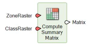
Compute Summary Matrix returns a matrix containing a cross tabulation of the two input rasters. In the returned matrix, row-column position [i, j] contains the number of pixels that have value i in **ZoneRaster** and value j in **ClassRaster**. The values in **ZoneRaster** are referred to as zones and the values in **ClassRaster** as classes.
