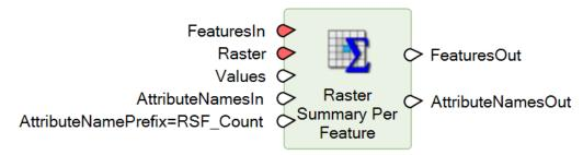
This operator computes the count of each DN value of the pixels of the input raster that are contained within a feature geometry (using the Primary Geometry field). The computed counts are added as attributes to the feature stream, one per value discovered in the input raster. The attributes are named by combining the value held by port **AttributeNamePrefix** and "<N>" where N is the pixel value. For example, by default, the name of the first column is "RS\_Cnt1."
