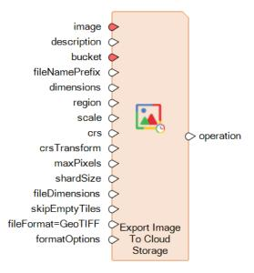
This operator lets you create a task to evaluate an Earth Engine Image expression and save it as one or more files in the named bucket in Google Cloud. The account to which the bucket belongs must have given access to the Earth Engine project being used.
