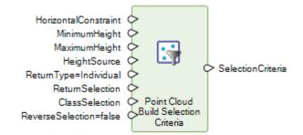
This operator enables you to define a set of selection criteria that can be used by other Point Cloud operators to define the points that they will operate upon. Several changes have been made for Update 2:
