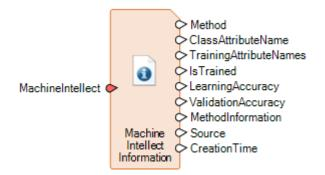
This operator provides basic information about a machine intellect and has been extended to provide information about imported deep learning models (see the Import operators detailed below.)
