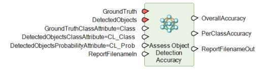
The Assess Object Detection Accuracy operator has been modified to take a list of features (since the Detect Objects Using Deep Learning operator now can generate a list of features and Assess Object Detection Accuracy needs to work through the list).
