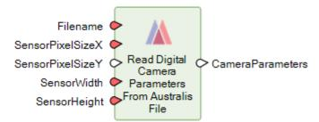
This operator reads digital camera parameters needed for setting up a Digital Camera from an Australis camera file.
