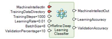
This operator refines the training on an existing deep learning classifier by supplying more training samples. This can be used to improve the overall accuracy or to tailor training for a new environment. The classes and band count in the training data must match the input machine intellect.
