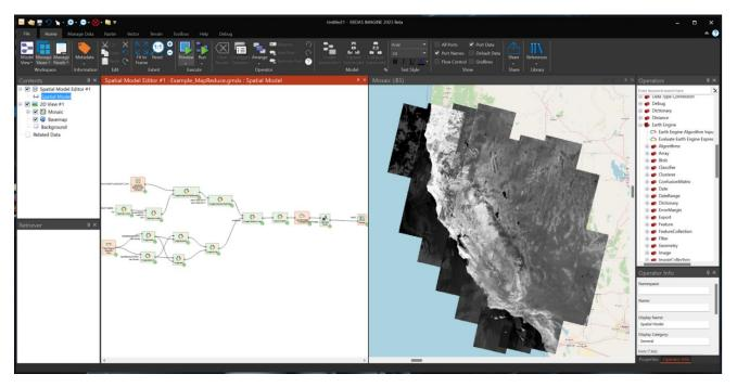
The screenshot above shows a spatial-temporal query being used to select all the images within a 600-km radius of San Francisco in 2022, the NDVI computed for each, and all combined into a single output. Just locating and acquiring all this data would have been a large, time-consuming task in the past.
