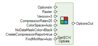
This operator creates the format-specific output-option dictionary for Enhanced Compressed Wavelet (ECW) format. This can then be fed to the Raster Output operator to control how an output ECW file might be generated.
