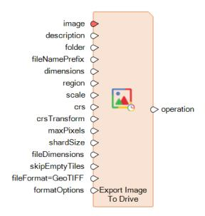
This operator lets you create a task to evaluate an Earth Engine Image expression and save it as one or more files in the named folder in Google Drive. The account folder must be accessible to the Earth Engine project being used.
