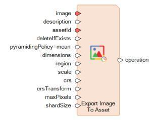
This operator lets you create a task to evaluate an Earth Engine Image expression and save the results as an asset in the Earth Engine Project space. Assets in the Project space can be directly used in further Earth Engine computations. The resulting asset ID is visible in the Project folder in the Earth Engine Catalog Browser.
