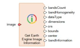
This operator evaluates the Earth Engine Image expression given on the **image** port and returns several pieces of useful information about the first band of the resulting image. Earth Engine images are not constrained to have homogenous bands. The outputs **dataType**, **dimensions**, **crs**, **bounds** and **center** are presented for the first band only, given that typically the bands are homogenous; however, the full set of metadata is returned on the **bandInformation** port.
