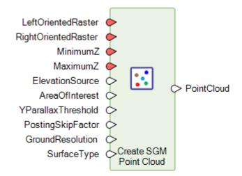
This operator extracts a point cloud from a stereo image pair using Semi-Global Matching (SGM) and saves it to an output point cloud.
