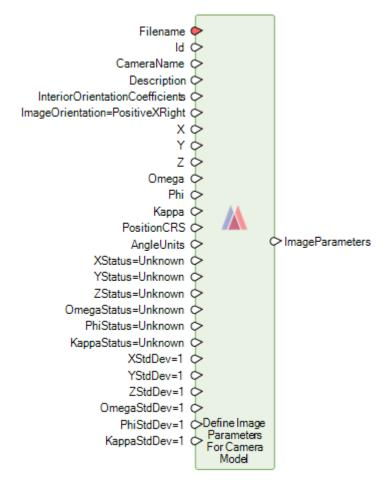
This operator creates a set of image parameters that are used when adding a camera sensor model to an image.
