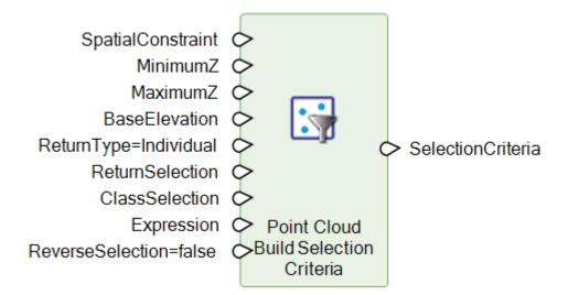
In order to simplify the process of setting **MinimumZ/MaximumZ** ranges specific to each **SpatialConstraint** geometry, the Point Cloud Build Selection Criteria operator has been enhanced.
