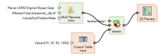
Since we want to iterate on the list of six TIFF files generated by the Multi Filename Input operator we make another connection from its output port to the IterationData1 port.
