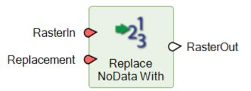
Replace NoData With no longer attempts to fill beyond the image's extent with the replacement value(s), i.e., outside the image remains NoData. This provides for more consistent processing when multiple datasets are being processed that have differing geospatial extents.
