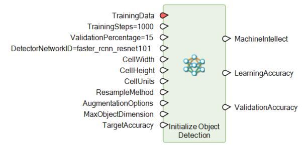
Initialize Object Detection now has a user-definable accuracy threshold at which to cease iterations.
