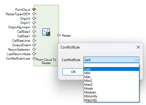
A **ConflictRule** port has been added to avoid "random" results when converting a point cloud to a raster. Previously for each output pixel, the last input point encountered which falls inside that pixel extent would be
