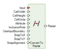
Convert To Raster rasterizes its input data at the specified resolution. In the case of Features input, a specific attribute field may be used to fill the rasterized geometries.
