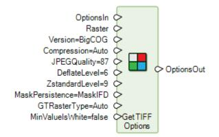
The Get TIFF Options operator has been updated in several ways to provide additional control over the formatting of downstream Raster Output operators which are set to produce TIFF formatted files.
