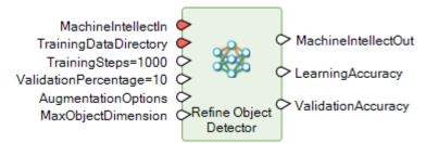
This operator refines an existing object detector by supplying more training samples. This can be used to improve the overall accuracy or to tailor the training for a new environment. The classes in the training data must match the input machine intellect.
