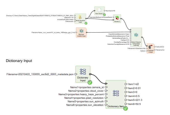
The Dictionary Input operator now reads JSON input files, which are sometimes supplied with satellite imagery to list metadata that can be useful in processing the data.
