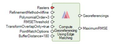
This operator accurately aligns the overlap area between adjacent georeferenced rasters to each other using edge matching. This will generate refined georeferencing for all rasters because the required shifts will be divided between the rasters. Edge matching may also be a good choice when the overlap area is small and it is undesirable to apply the same transform that is suitable for the overlap region to the entire raster.
