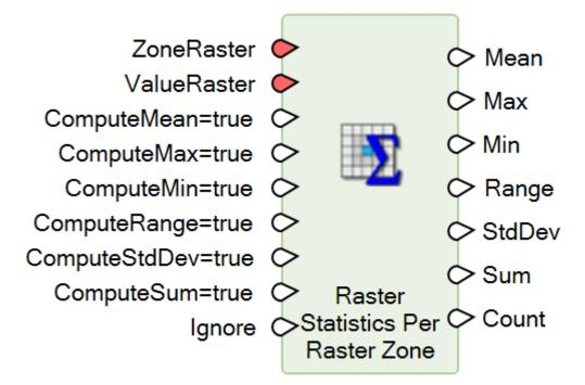
This operator computes selected statistical measures of all pixel DN values from **ValueRaster** that are overlaid by each zone (i.e., DN value) of **ZoneRaster**. Row i of the returned Table contains the statistical measure from **ValueRaster** of all pixels that have value i in **ZoneRaster**. By default, all supported statistics are computed and output.
