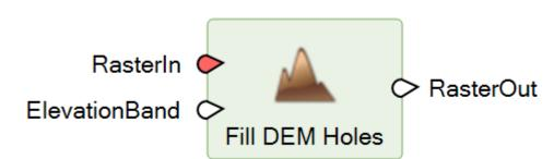
The operator identifies NoData pixels or areas, otherwise known as holes, in the input raster. It uses TIN interpolation between pixels that border the NoData areas, to determine the DN values used to update NoData pixels. Only NoData pixels within the convex hull of the TIN are modified. All other pixel DN values are passed through unchanged.
