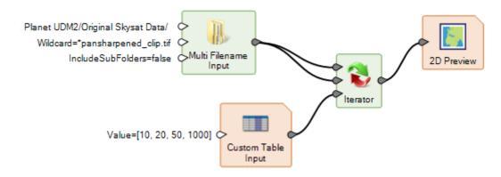
Now the model has been told to iterate using the list of six TIFF files. Consequently, for each of those raster images the sub-model inside the Iterator will add 10 to the DN values of band 1, 20 to band 2, 50 to band 3 and 1000 to band 4, as originally desired.
