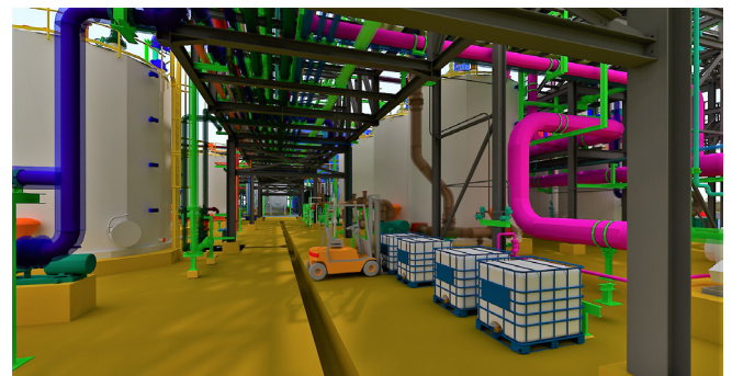
A rendered view of the 3D model showing some details such as piping, equipments, steel structure, supports and secondary steel that's created with CADWorx.
