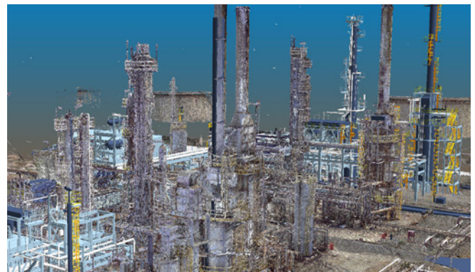
Figure 2: a view of the new objects and a point cloud of the existing plant.
