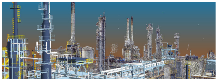
Figure 1: a view of the new objects to be built from Intergraph Smart 3D combined with a point cloud of the existing plant.
