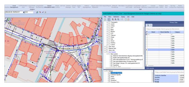
A municipality's underground electrical, telecommunication and water/wastewater networks are shown in one view in HxGN NetWorks Utilities.
