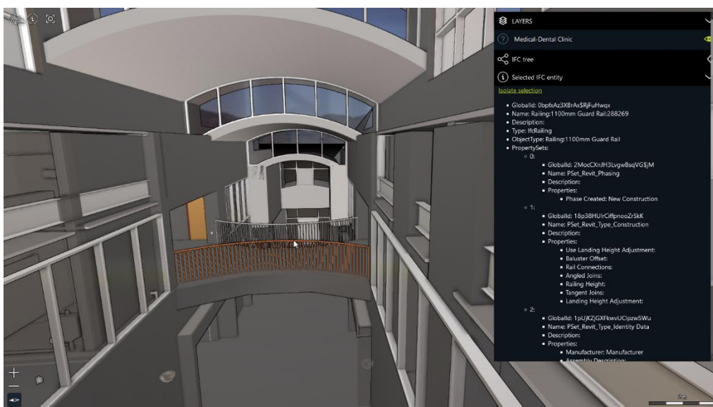
Figure 2: IFC data visualized in LuciadRIA, delivered via LuciadFusion, showing the properties of the selected element
