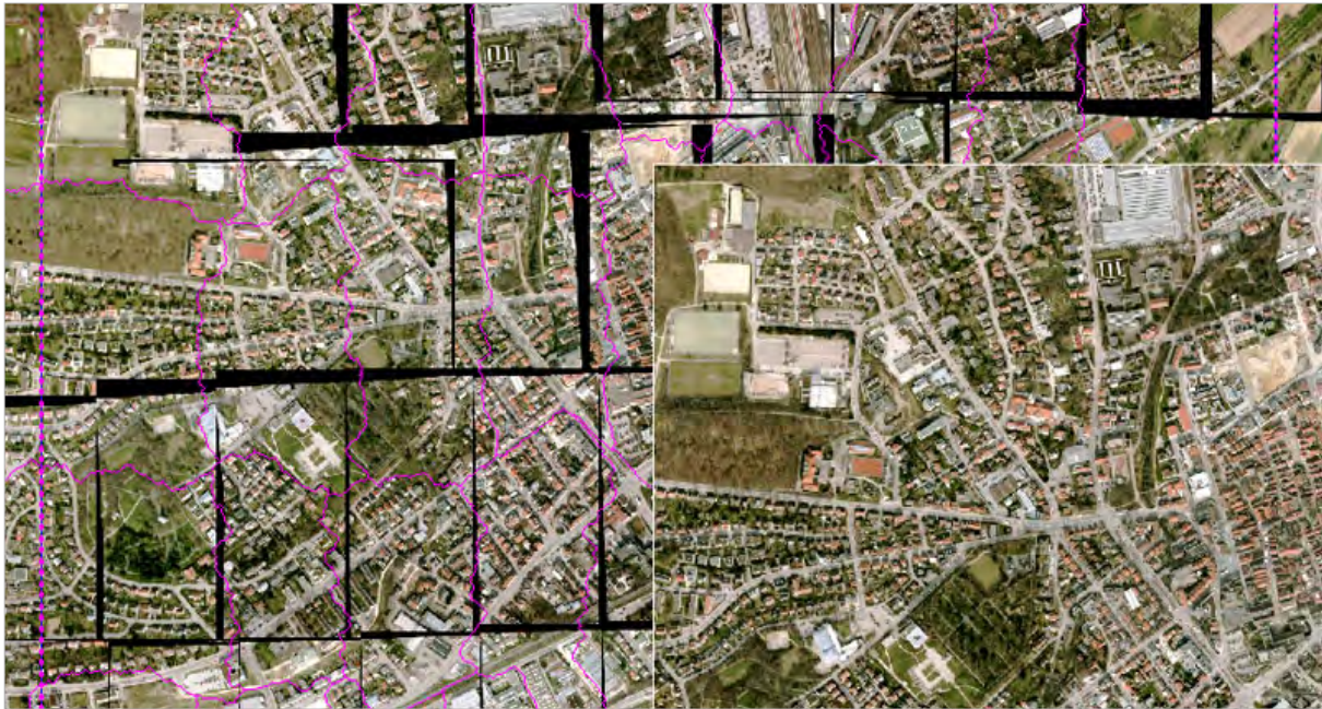
ImageStation OrthoPro provides a complete solution for orthorectification, enhancement, automatic seamline generation, tone balancing, and mosaicking.
