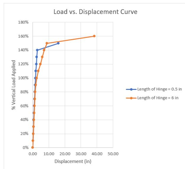
Let us now examine this same beam with an axial load applied in addition to the load applied at node #2. The load vs. displacement curve for this case is shown below.
