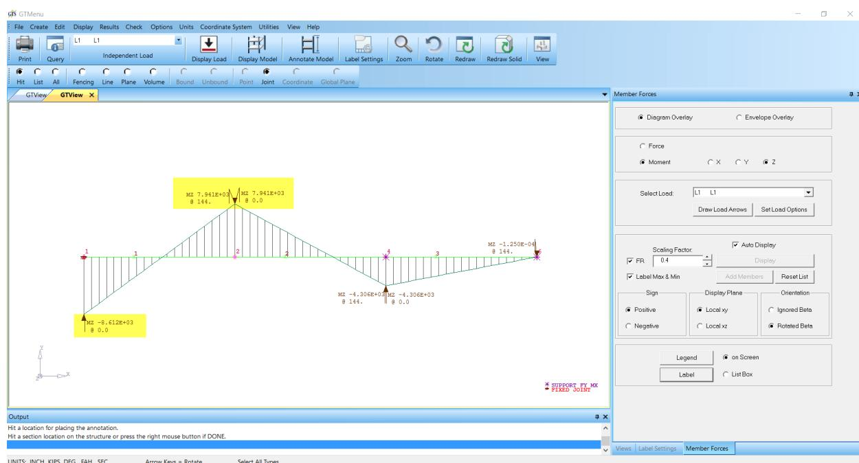
However, we do not have the ability to do a code check in a real structures lab. In a structures lab, we need to establish failure criteria. If this beam were loaded with 200 kips of loading in a structures lab, we would see a catastrophic failure of the beam. This failure most likely will have the formation of plastic zones.
