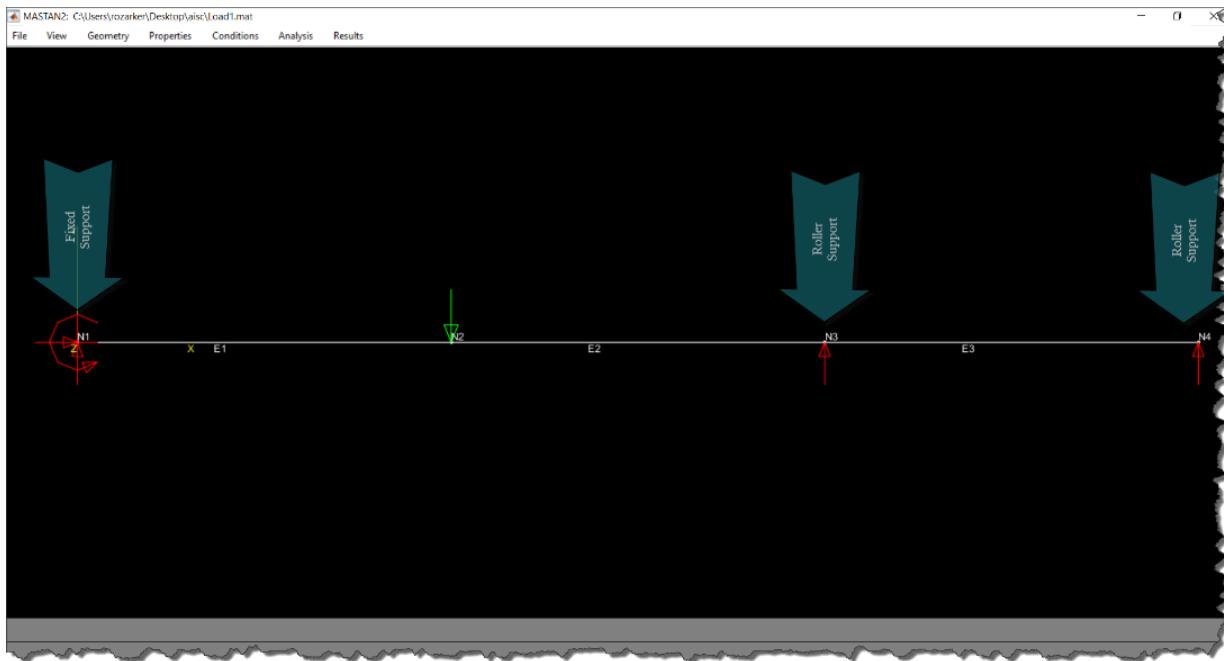
First, let us load the beam with a 100-kip unit load.
