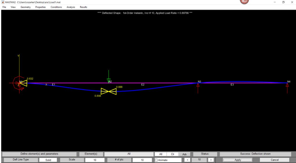
GT STRUDL also offers the option for users to define the length of the plastic hinge, which will affect the displacement results. A beam with a larger plastic zone will deflect more than a beam with a smaller hinge length as shown in the following table.
