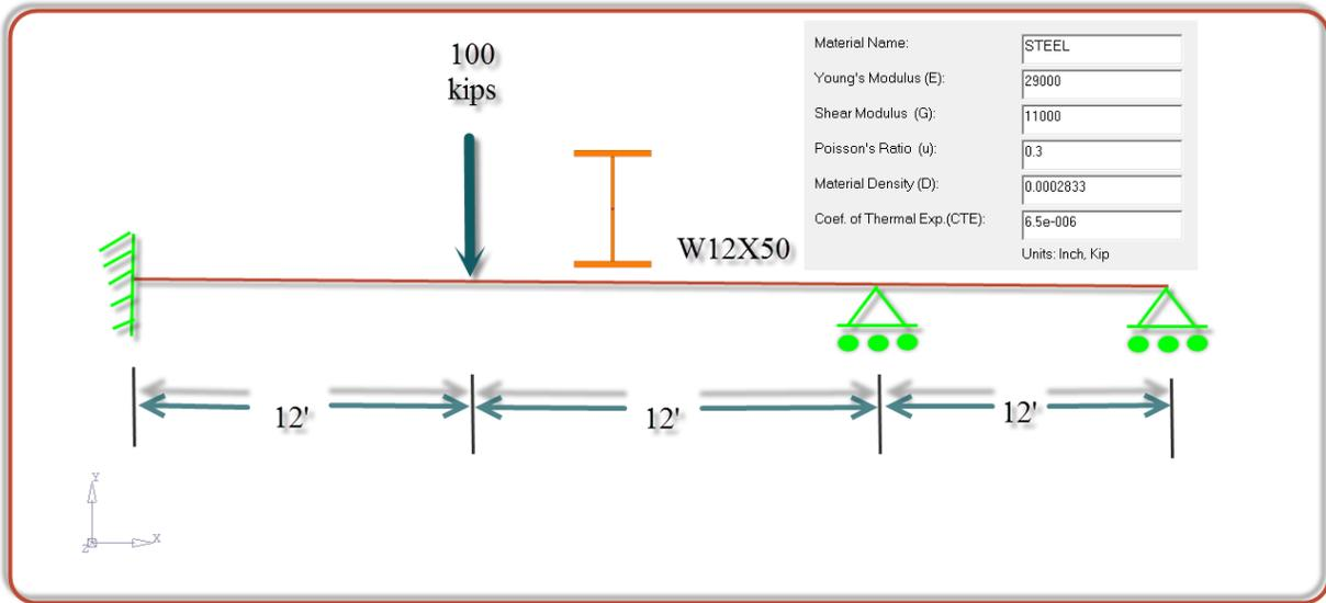
Looking at the results of this unit load, we see a 1.58" deflection at node 2, the point of load application.
