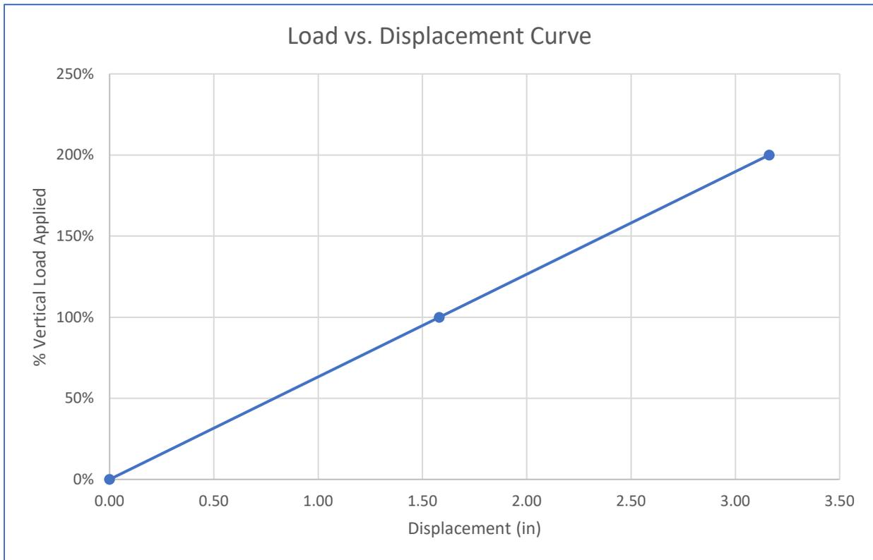
This means that while the beam will eventually fail a code check, it will continue to have linear displacements as the load increases well beyond the code allowable load.
