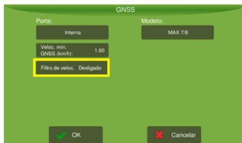
Figure - Speed filter
