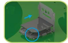
Figure - SIM card housing step 1
