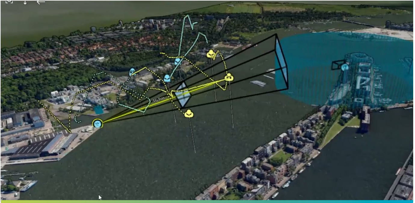
Example of multiple sensor feeds, including AI classified drone tracks, radar responses and video feeds over a demonstration area
