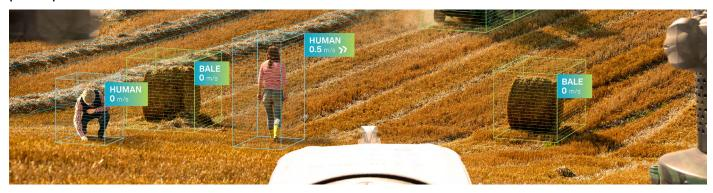
Enable automation and ADAS in agricultural applications with Hexagon Autonomy and Positioning Perception solution. The kit contains ECU, four surround-view mono cameras, stereo camera with cables and brackets to get you started. Together they provide an accurate and robust solution for positioning objects and obstacles around the vehicle with Hexagon's robust agriculture specific algorithms.
