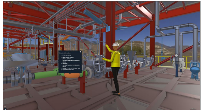
Figure 8: Monitor editable building information through selection and expression-based styling on 3D data.
