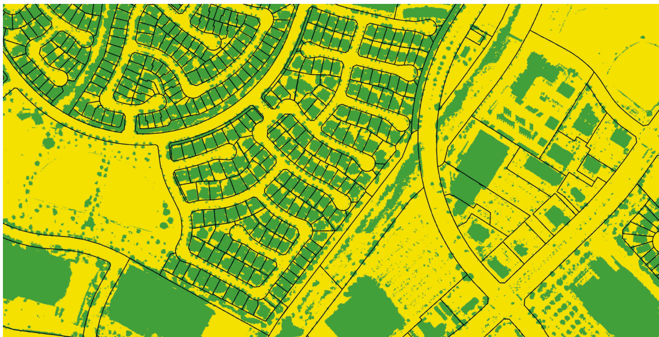
Figure 4. The model applied a height filter using DSM data where the yellow areas represent land cover under 5 feet and the green areas show greater than 5 feet. (Source: DCSE, Inc.)
