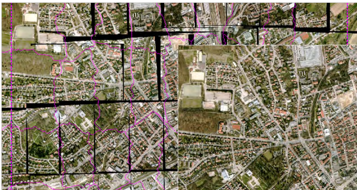
ImageStation OrthoPro provides a complete solution for orthorectification, enhancement, automatic seamline generation, tone balancing, and mosaicking.
