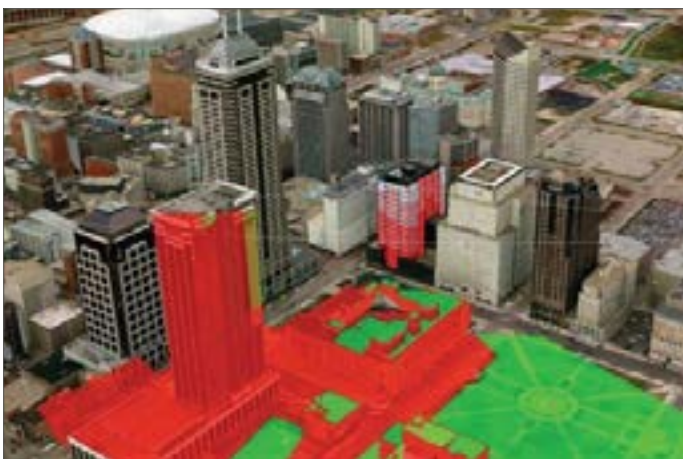
GeoMedia 3D quickly runs a viewshed analysis from any selected point on high-rise buildings that can more accurately justify increased/decreased valuation based on various views.
