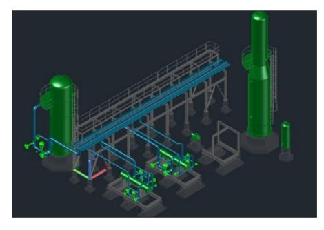
Figure 4: This CADWorx model shows .dwg files referenced in AutoCAD to create a single view of the plant.
