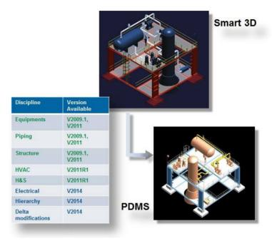
Figure 7: Smart 3D exports designs and catalog data for most disciplines used by PDMS.
