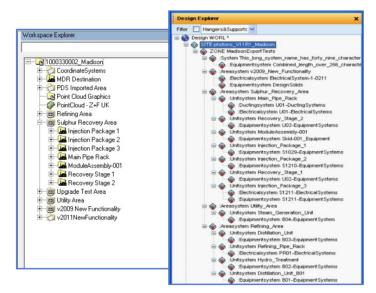
Figure 8: The plant hierarchy is incrementally mapped to PDMS schema types.
