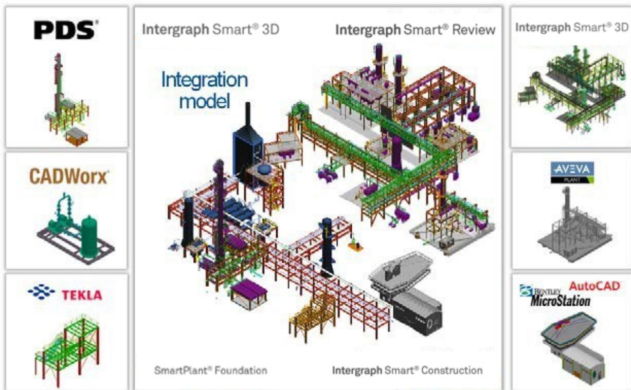
Figure 1. Hexagon PPM's interoperability technology incorporates designs and data from many sources.
