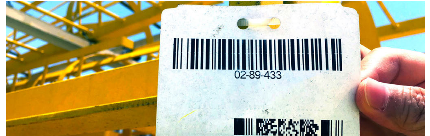
Passive RFID tags and vendor-supplied barcodes are associated to finished materials at supplier and fabrication facilities.
