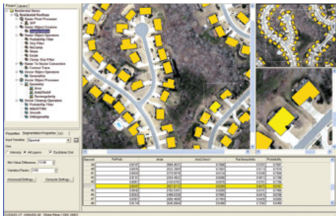
The IMAGINE Objective workspace shows a feature model designed to extract the locations of building footprints in a GIS-ready form to minimize manual post-processing and editing.
